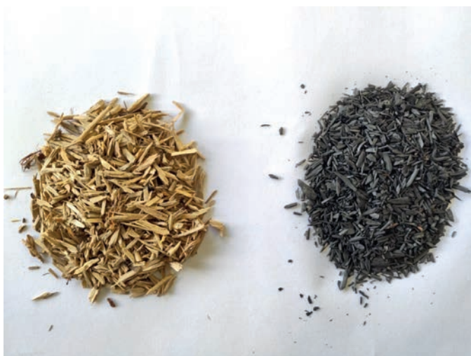
Substrate – crushed garden waste and the product - biochar
